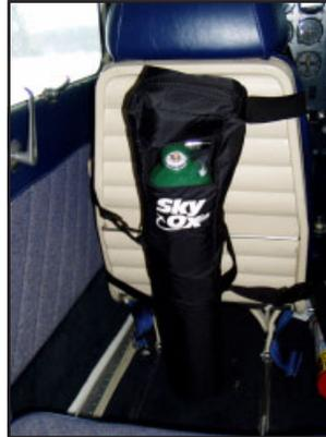
**Reminder:** The system is under 2000 pounds of pressure when full. As a safety measure, the regulator is equipped with a pressure relief valve that's designed to activate under a reduced pressure rate to depressurize the tank.
